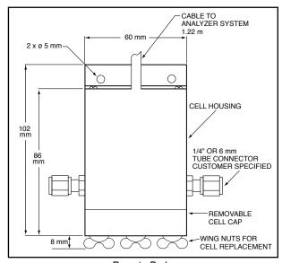
Remote Probe Housing 60 mm x 102 mm H x 62mm D
